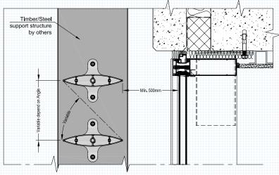
30° Large blades allow for larger gaps between the blades, ensuring excellent transparency with sufficient light for the building
